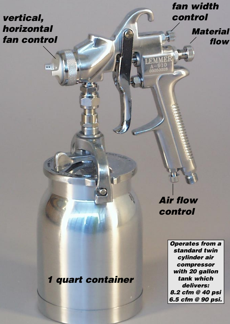
L015-012 conventional 1.8 spray gun with suction pot (shown) L015-013 pressure feed 1.4 mm version (without container)
