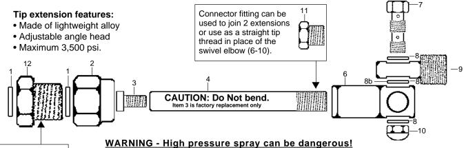
Tip thread adapter on this end for Lemmer equipment. For Graco equipment move this adapter to the other end. • Read spray pump operating manual and safety instructions.
