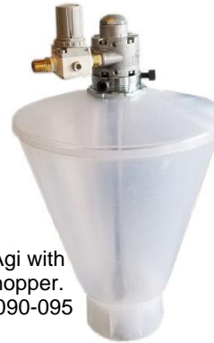
1/3 HP agitator mount for 2" bung or any port hole. Zinc plated steel construction. Parts shown: L090-053 bung adapter L090-075 bung nut, each L002-781 bolt 5/16x1" soc L005-743 bolt 5/16x3/4" hx
