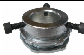
1/3 HP agitator mount for 2" bung or any port hole. Zinc plated steel construction. Parts shown: L090-053 bung adapter L090-075 bung nut, each L002-781 bolt 5/16x1" soc L005-743 bolt 5/16x3/4" hx
