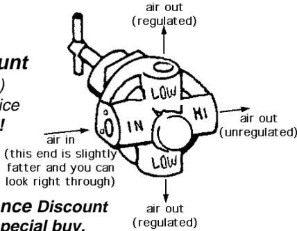
**Air regulator.** Flow through design has one unregulated air out port, 2 regulated out ports. This design is used on some pressure pots to allow unregulated air to go straight through to the gun air cap while it regulates the air going to the pot. Steel T-handle is lockable. All ports are 1/4" npt. Available in 2 pressures as listed below.
